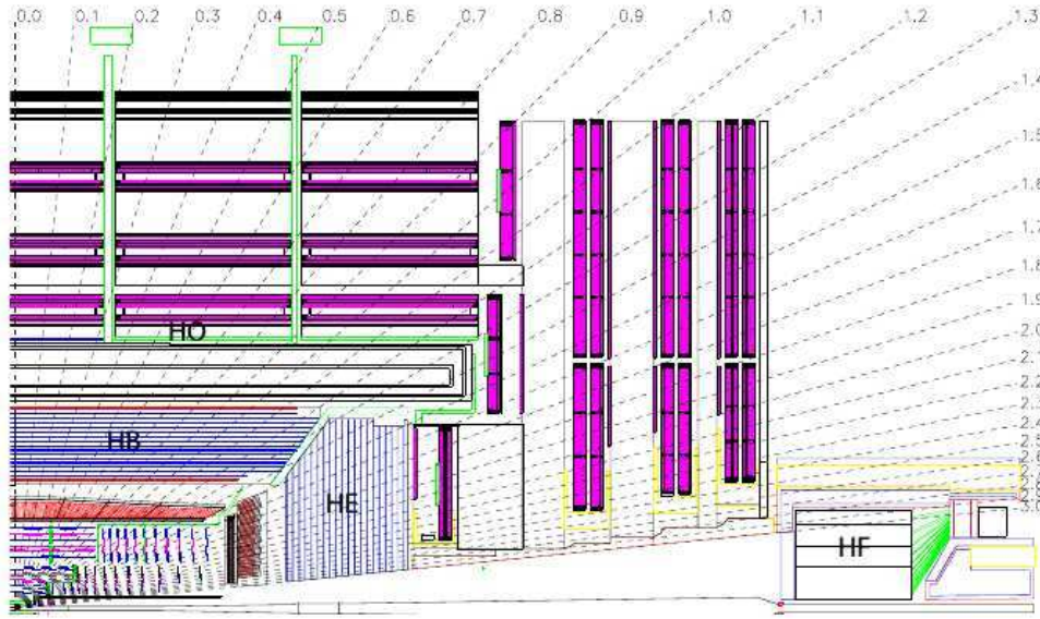
Figure 10: Longitudinal view of CMS showing HCAL.
