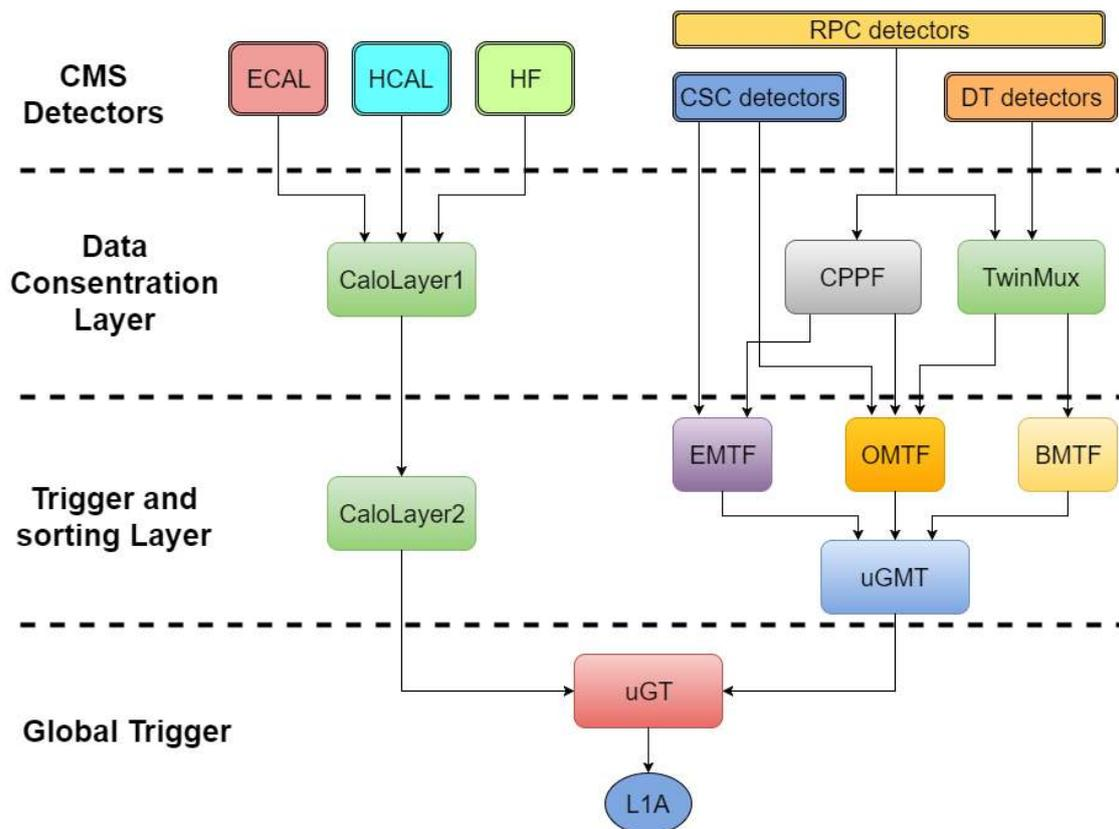
Figure 3.2: The upgraded L1 Trigger architecture and data flow of CMS
