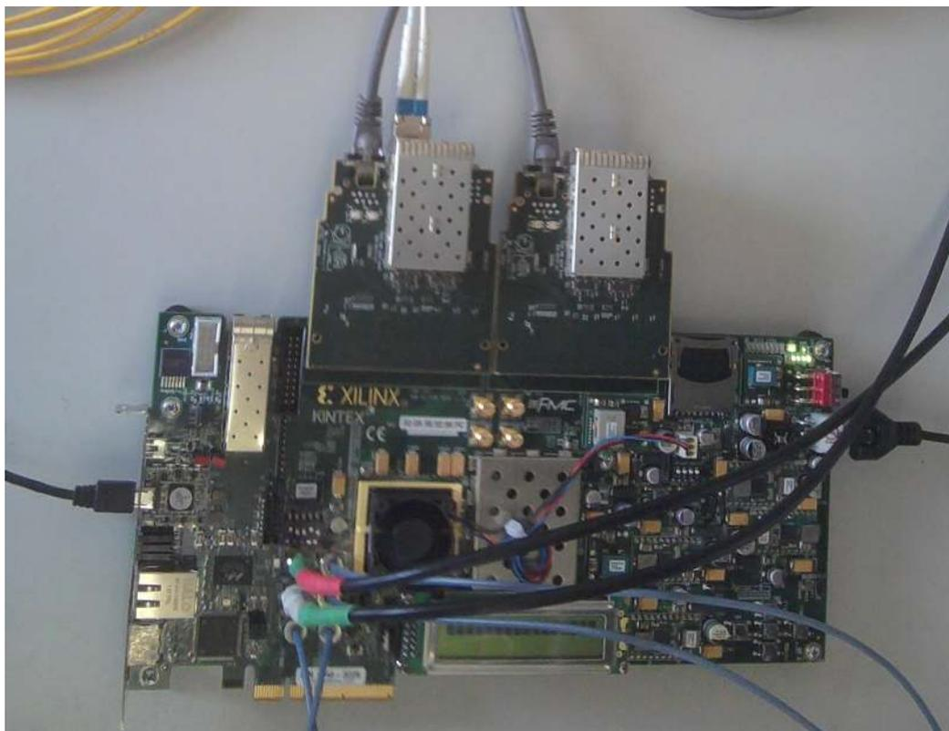
Figure A.8: Two EDA-02727-V1 mounted in the KC705 development card
