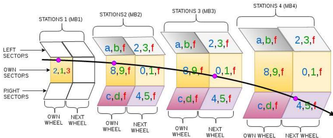
Figure 4.7: A muon that gives the track address 0x2804. This muon leaves signal in own sector - own wheel - station 1, own sector - own wheel - station 2, own sector - next wheel - station 3, right sector - next wheel - station 4. In this example the track segments are exclusively from the TS1.
