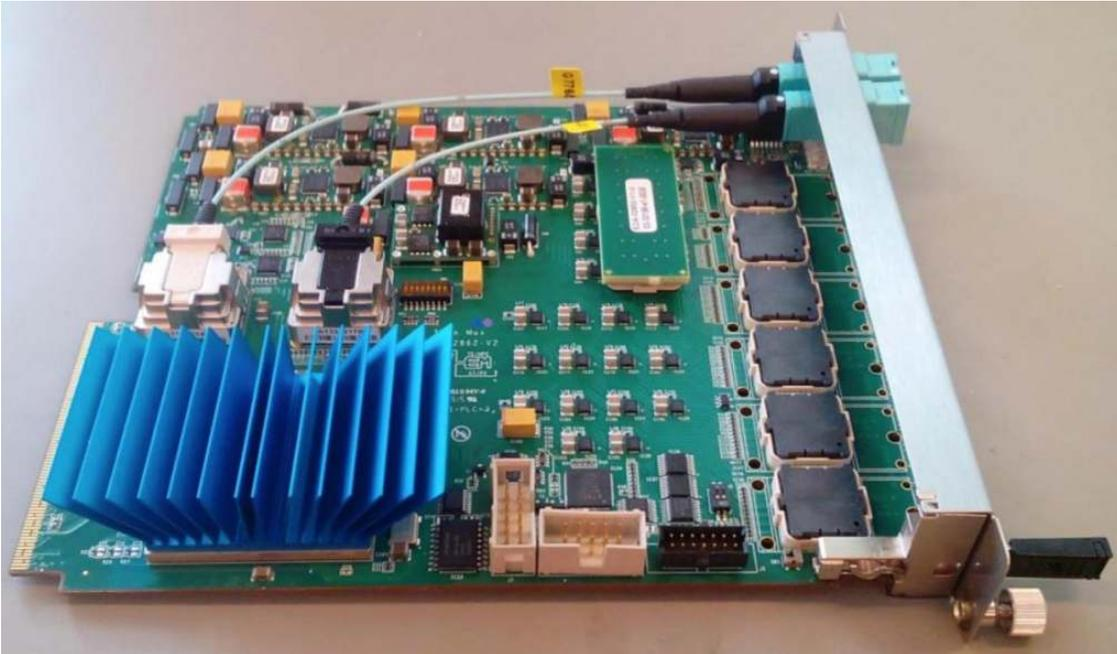
Figure 3.9: The TwinMux card. This AMC card uses a Virtex-7 FPGA that pre-processes TPs and transmits them to the track finders using optical links.
