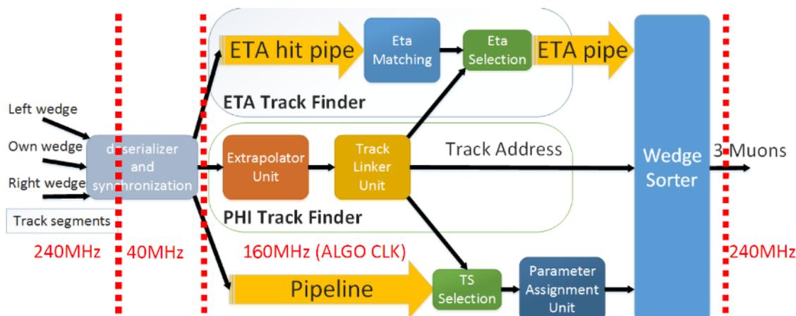
Figure 4.18: The BMTF algorithm blocks, divided in three different clock domains: The 240-MHz domain where the 10-Gb/s links are implemented, the 40-MHz domain where the input data are formatted and concentrated and formed and the 160 MHz where the BMTF algorithm is running.
