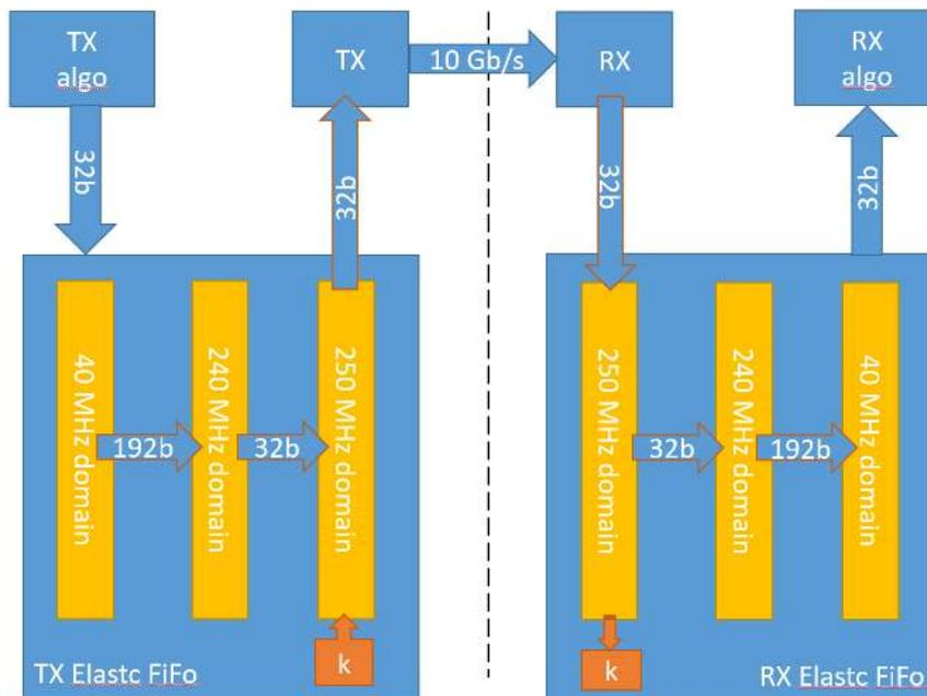
Figure F.2: Block diagram of the asynchronous protocol 10 Gb/s
