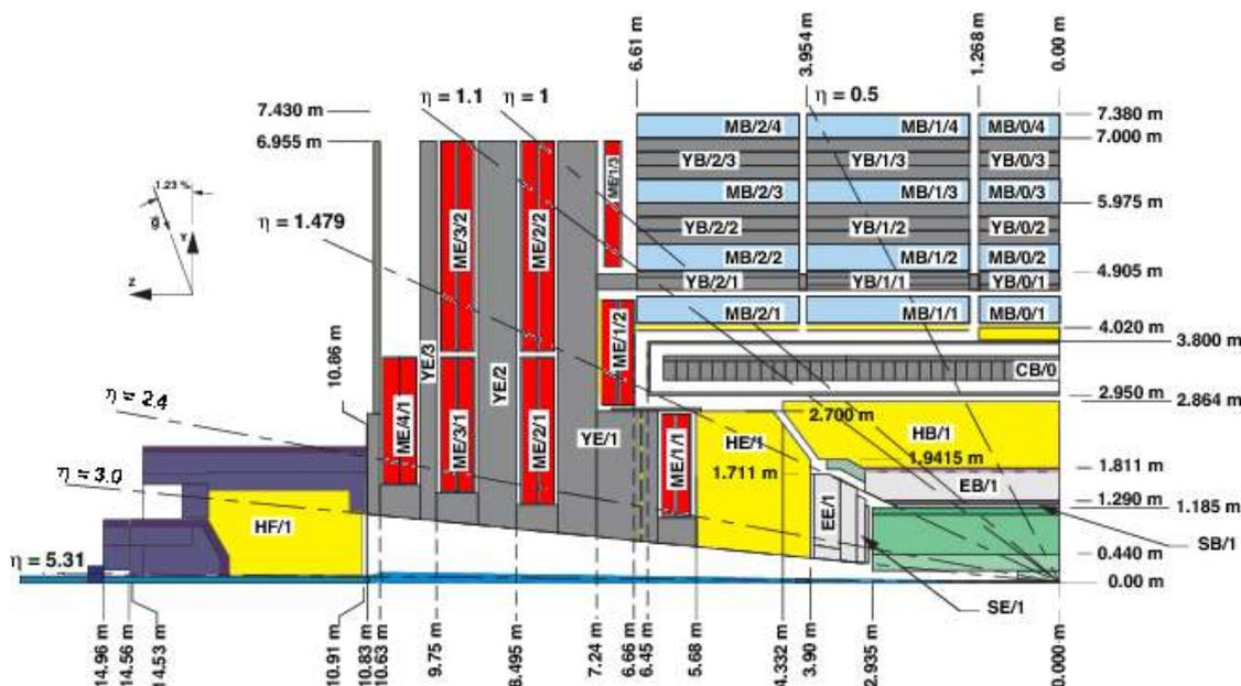
Figure 2.14: Schematic view of one quarter of CMS, in the  $z-\phi$  plane. CSC chambers appear with red color.
