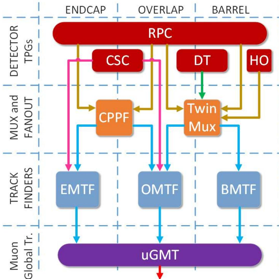
Figure 3.8: The L1 Muon Trigger architecture of CMS after the phase I upgrade. The color of the arrows indicates the transmission protocols used with optical links. Green: synchronous 480 Mb/s, Brown: synchronous 1.6 Gb/s (GOL links), Pink: synchronous 3.2 Gb/s and Blue: asynchronous with the LHC clock, 10-Gb/s links.
