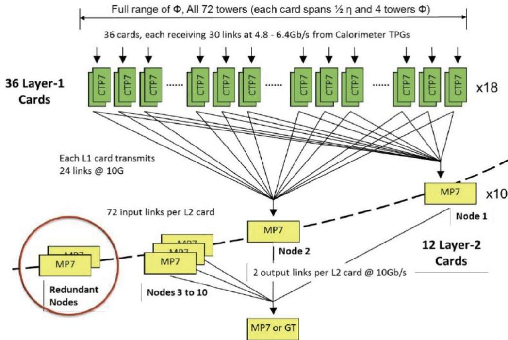
Figure 3.7: Time Multiplexer Trigger (TMT) architecture.
