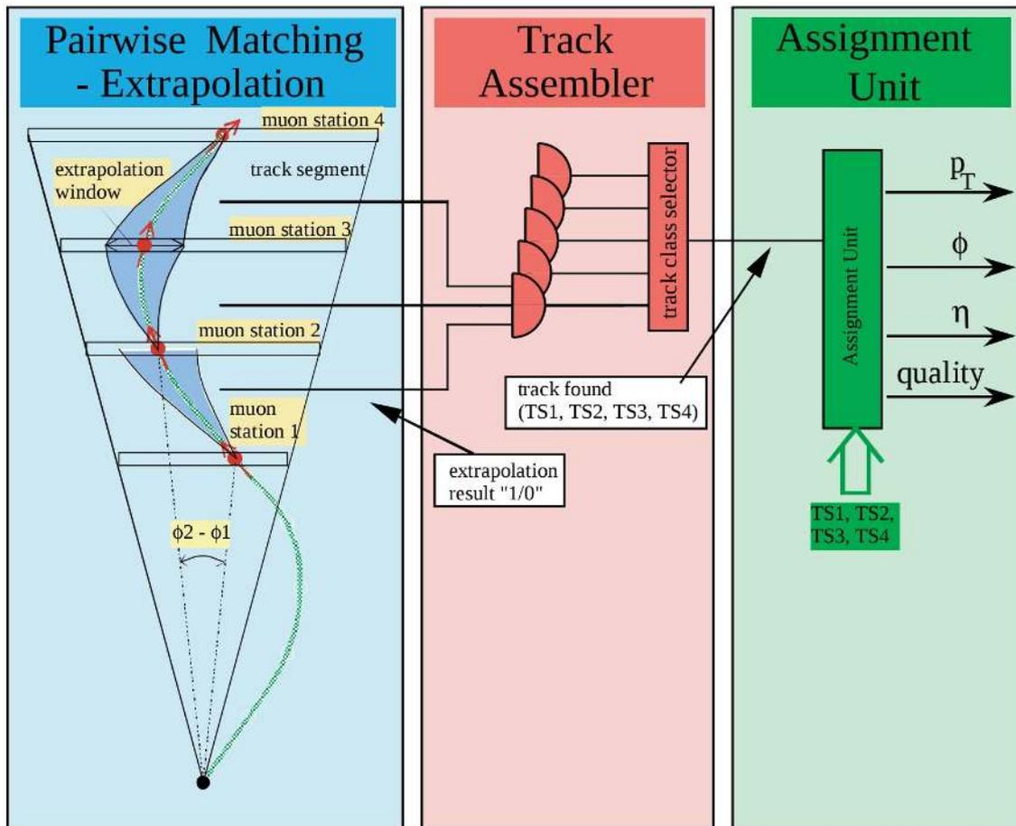
Figure 4.3: PHI Track finder and assignment unit
