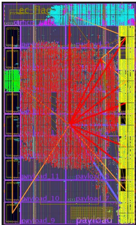
Figure 4.19: Implementation of the BMTF in the FPGA die.
