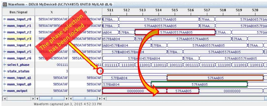
Figure 7.11: ISE Chipscope - Validation of the 40 Mb/s receiver block
