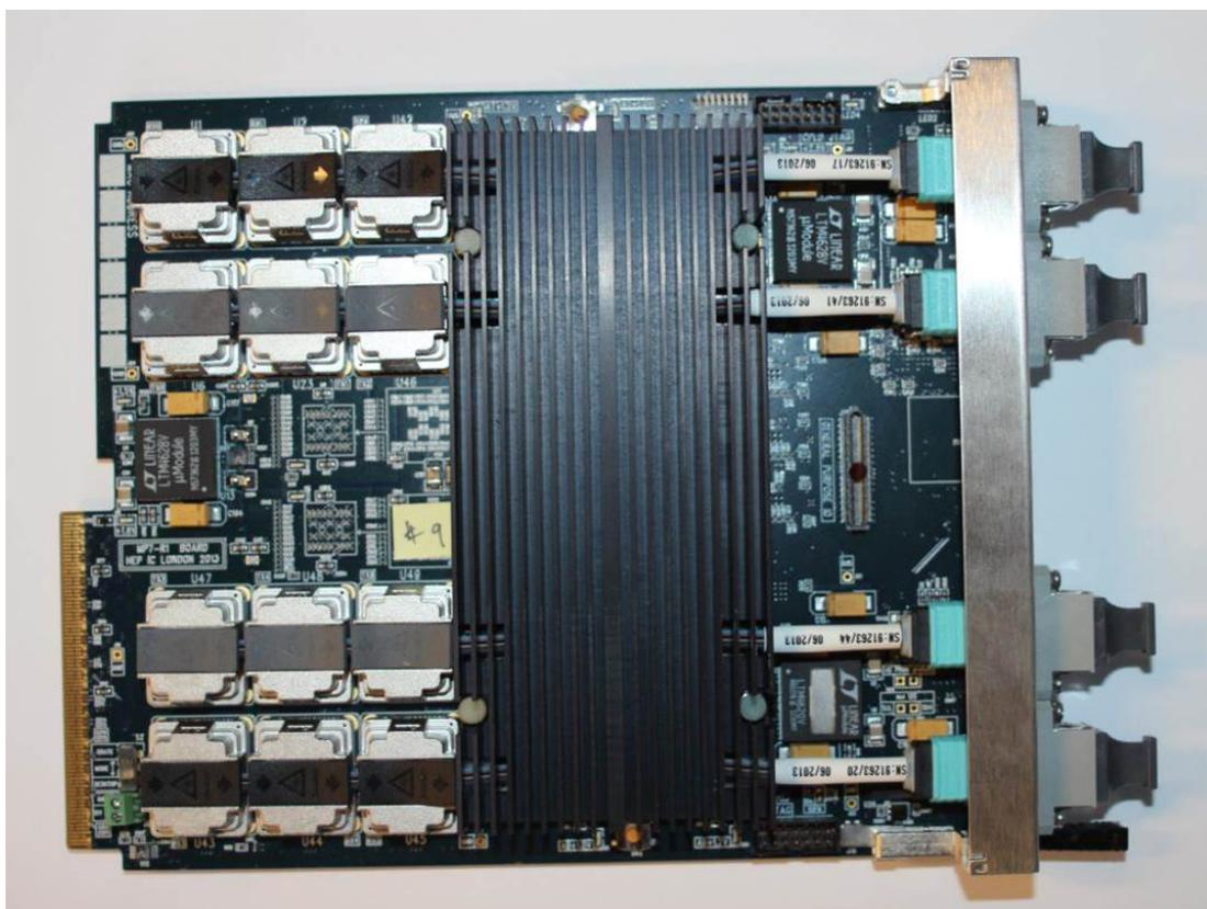
Figure 4.15: The XE type MP7 card is used in the BMTF system. 12 minipod optics (showing on the left side next to the heat exchanger) are connected via multimode fiber to 4 MTP connectors (front panel).
