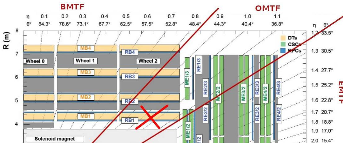
Figure 6.2: BMTF 1st stations of wheels  $|2|$  are masked during collisions.
