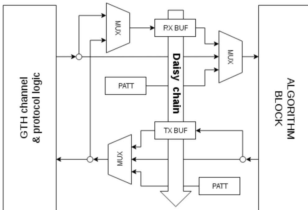
Figure 4.17: Block diagram of MP7 buffers and their configuration logic: The buffers (RX BUF, TX BUF) are 1024 long and 32-bits width. A set of multiplexers is controlled by the configuration and set the buffers in normal, test or DAQ mode. In normal mode the buffers capture data which pass though. In test mode the buffer are used to send data to the algorithm or to the optical links. In DAQ mode the buffers are connected in a daisy chain data flow and collect data to be sent through the DAQ.
