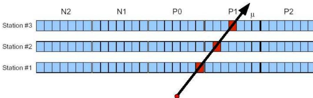
Figure 4.9: In a wedge of the muon chambers a muon hit: the seventh area of the station 1 in wheel 0, the second area of station 2 and the fourth area of station 3 in wheel 1. N2, N1, P0, P1 and P2 are sectors.
