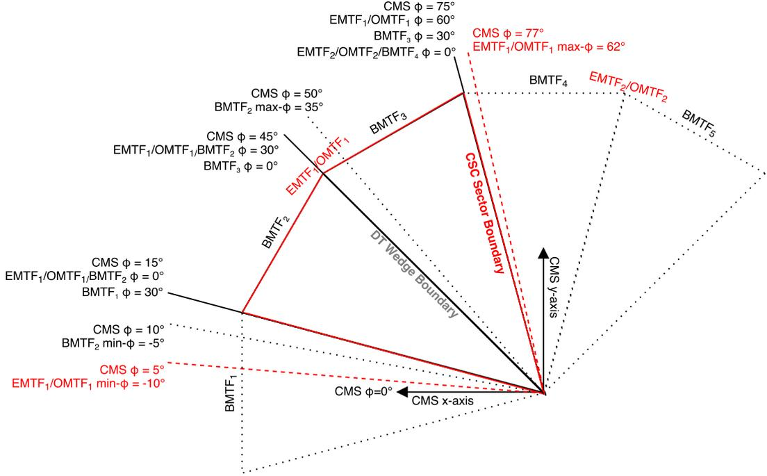
Figure C.2: Relative  $\phi$ -scale for the track finders starts counting at the edge of the processed wedge or sector. The range is different for BMTF as it processes  $30^\circ$  wedges, and OMTF/EMTF which process the  $60^\circ$  sectors.
