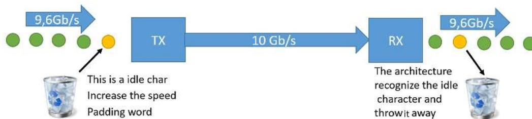
Figure F.1: 9.6-Gb/s asynchronous link
