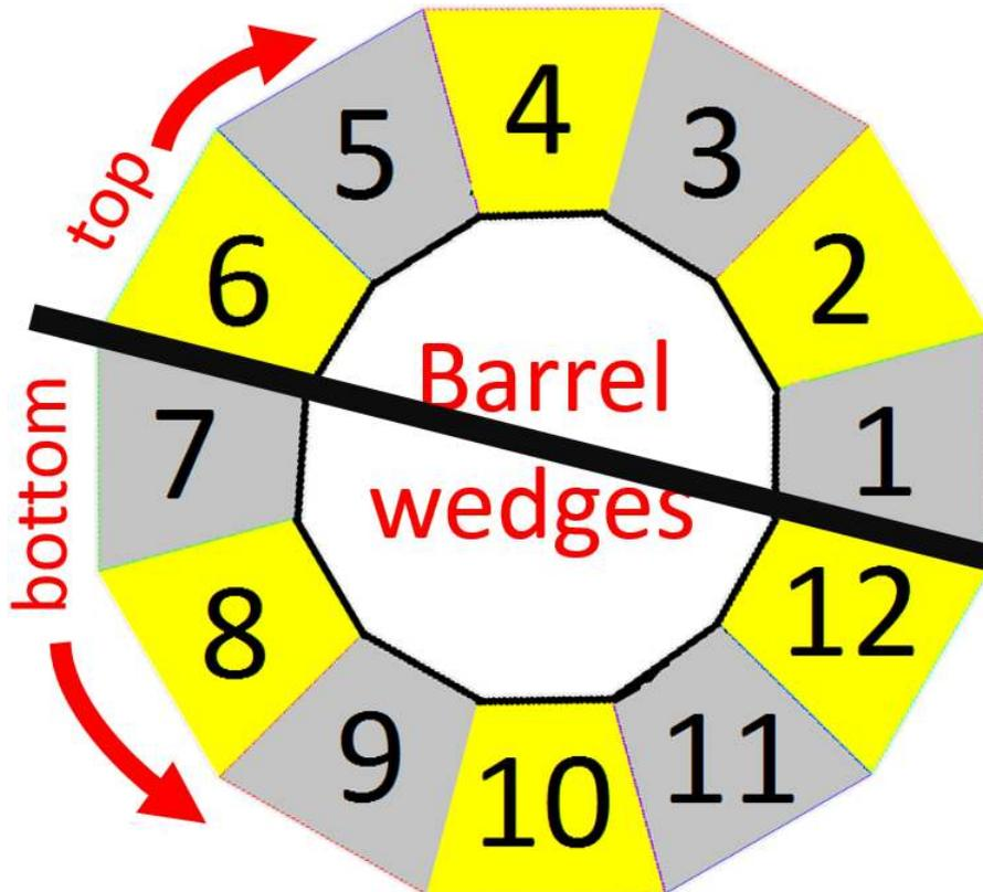
Figure 4.13: The BMTF system is splitted into two crates. The TOP includes the 1, 2, 3, 4, 5, 6 processors and the BOTTOM the 7, 8, 9, 10, 11, 12.
