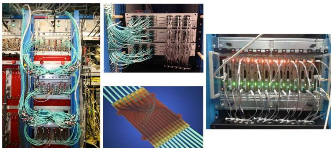
Figure 3.4: The Level-1 Trigger Calorimeter system. On the left is the CaloLayer1. On the right is the CaloLayer2. On the top middle is the patch panel. On the middle bottom is the Molex FlexPlane.
