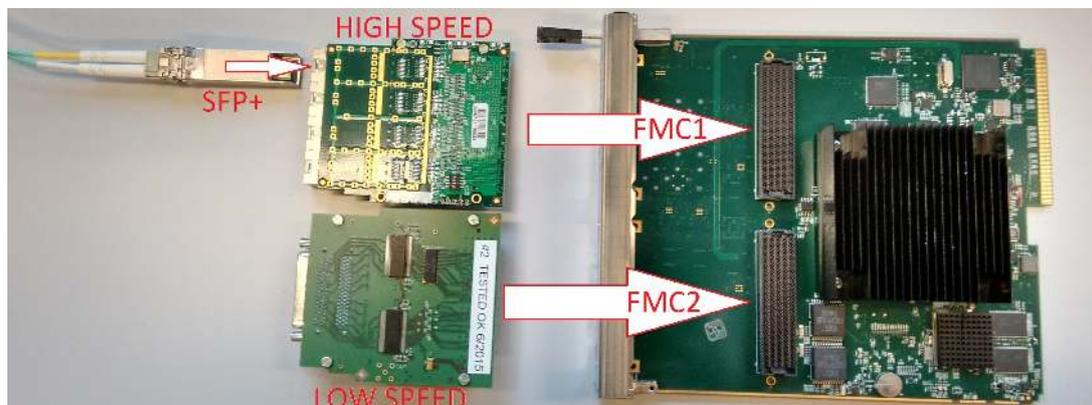
Figure 7.7: AMC502 card, the high and low speed mezzanine modules and the SFP+ optic
