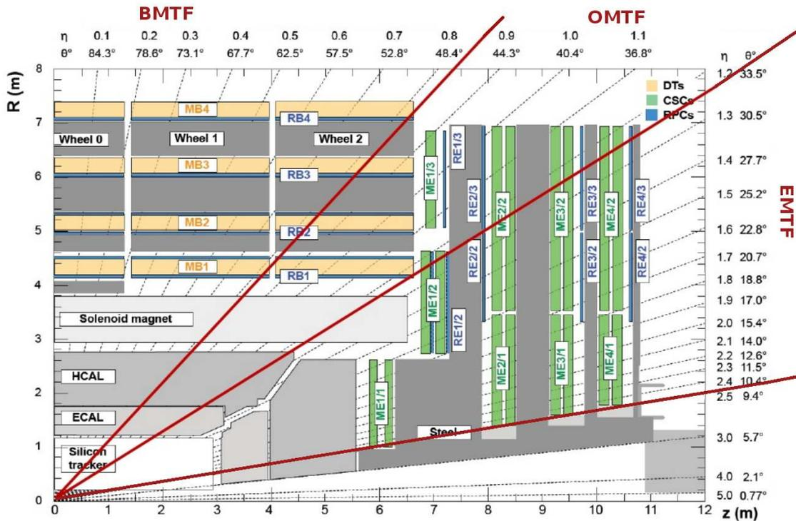
Figure 4.1: The longitudinal view of one quarter of CMS detector and the three muon track finder regions: BMTF, OMTF and EMTF.
