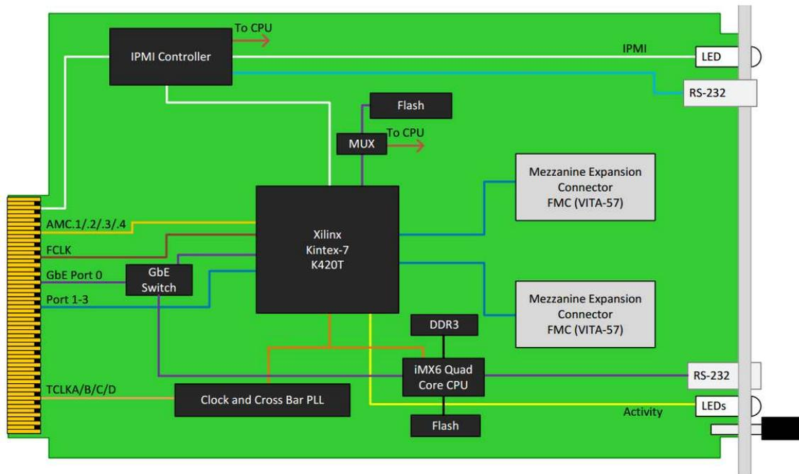
Figure 3.17: AMC502 block diagram.
