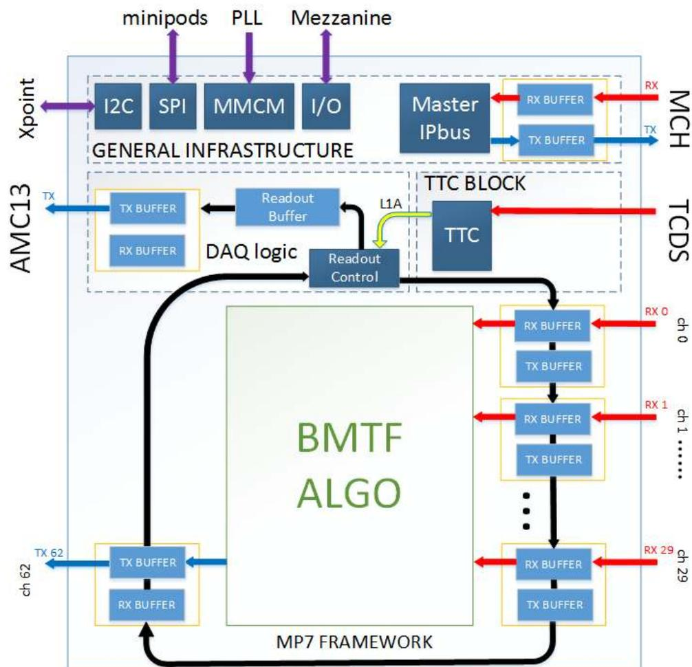
Figure 4.16: Block diagram of the BMTF firmware. The core of the logic is the BMTF algorithm and wrapped around the set of logic blocks (framework) that supports the core and implement all needed functions: serializes/deserializes, DAQ and TCDS interface, control of the system through ethernet (IPbus) and control of on-board components.
