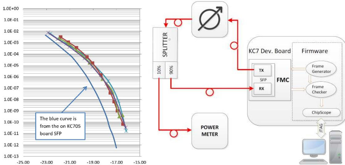
Figure A.3: Evaluation setup and BERT curves of F18 and EDA-02708-V1. Left: PCB performance - BERT curves. Y-axis represents the bit-error rate and X-axis the optical power in dbm. Right: Setup and logic for the evaluation test.
