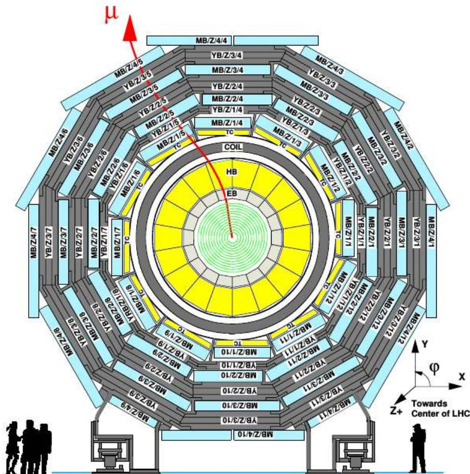
Figure 2.15: Schematic view of one of the five wheels of the barrel of the CMS experiment, in the x-y plane and a track of a muon.
