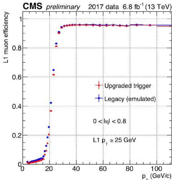
Figure 5.15: Barrel (BMTF) and legacy (DTTF) single Muon efficiency versus  $p_T$ .
