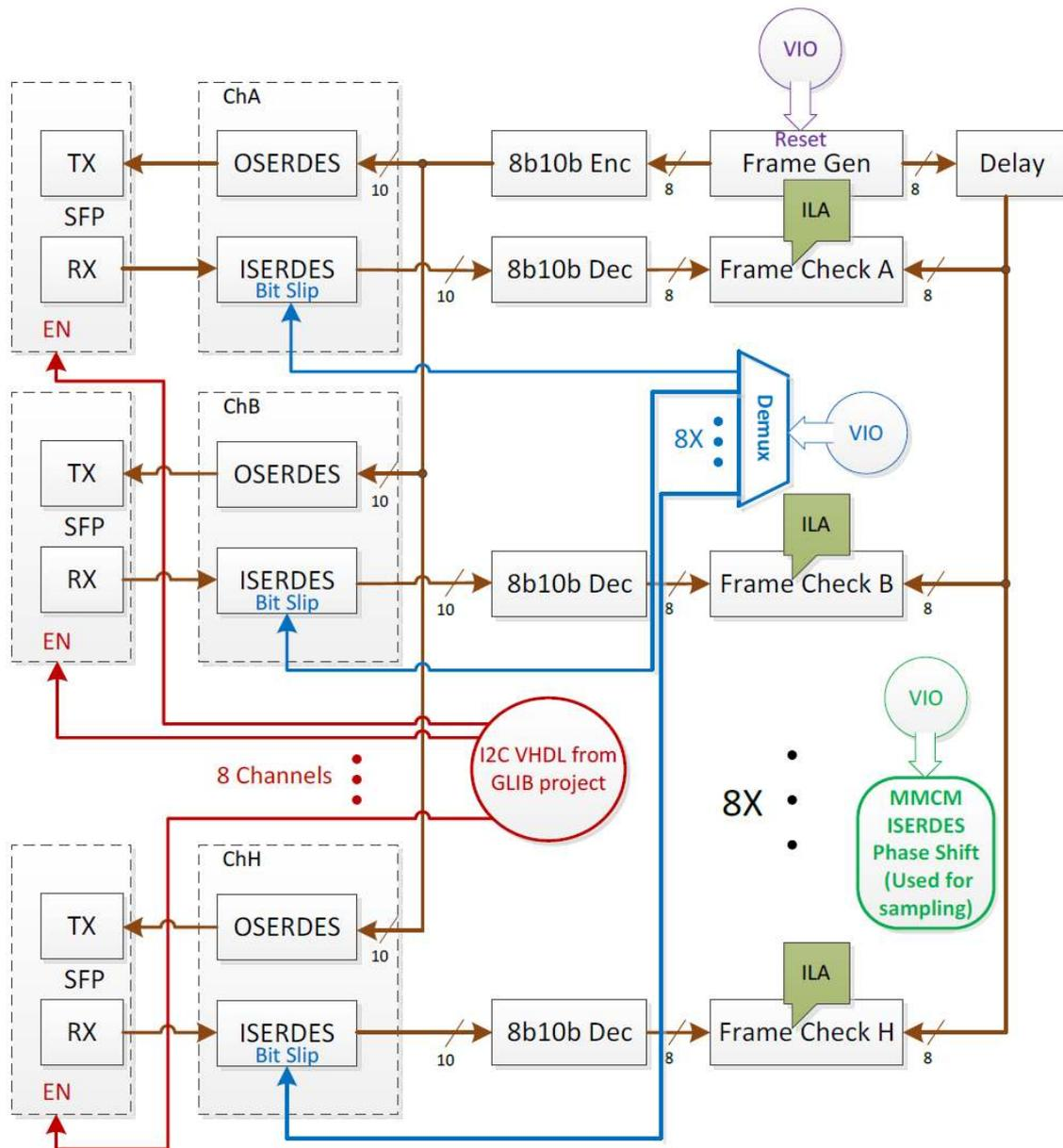
Figure A.5: VHDL block diagram used to evaluate EDA-02707-V1
