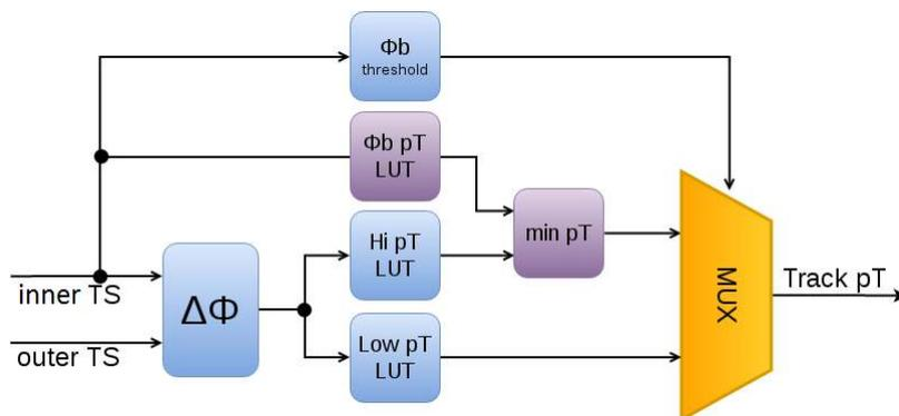
Figure 4.8: The assignment algorithm. The blocks in blue are parts of the old algorithm and in purple of the new algorithm. The  $p_T$  assignment is calculated either using the  $\phi$  difference between the inner and the outer stations or by the  $\phi_b$  of the inner station.
