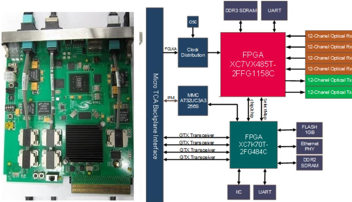
Figure 3.12: The hardware of the Concentration Pre-Processing and Fan-out card. Left: CPPF card. Right: CPPF block diagram
