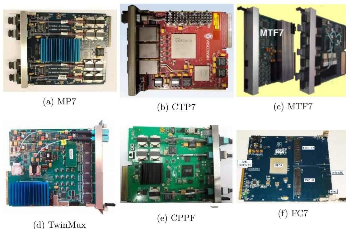
Figure 2.16: AMCs used in CMS for the phase I trigger upgrade
