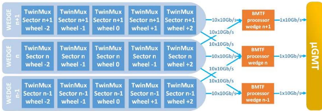
Figure 4.11: Distribution of input data primitives to the BMTF processor and output triggered data from the BMTF processor. With blue color the Twinmux cards, with orange the BMTF and with yellow the  $\mu$ GMT (both MP7s) are shown.
