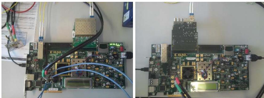
Figure A.2: KC705 used as the carrier platform testing the FMC cards. Left: Faster Technology F18 on KC705 platform, right: EDA-02708-V1 on KC705 platform.
