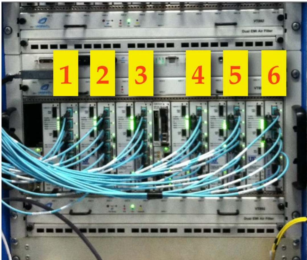
Figure 3.15: EMTF crate. It hosts six dual MTF7 modular platforms including one base card, one optical card and one LUT mezzanine. The optical cards are connected with multimode fibers operating up to 10 Gb/s.
