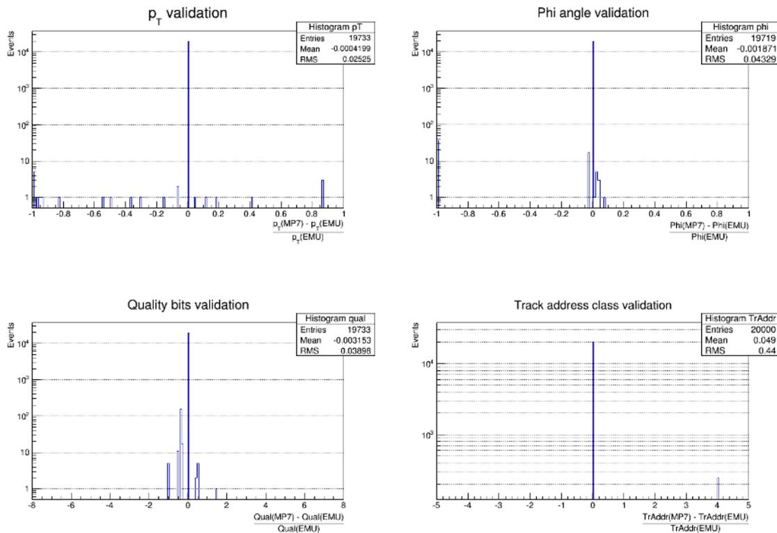
Figure 5.2: Histograms of hardware algorithm output compared with emulator output ( $p_T$ ,  $\phi$ , quality bits and track addresses). Magnitude:  $\frac{X_{MP7} - X_{EMU}}{X_{EMU}}$ , where X:  $p_T$ ,  $\phi$ , *Quality bits*, *Track Address*
