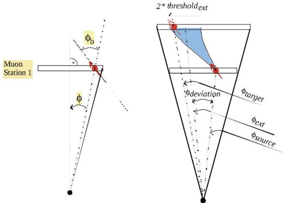
Figure 4.4: Extrapolation parameters. Left:  $\phi$  and  $\phi_b$  angles, right:  $\phi_{source}$ ,  $\phi_{extrapolated}$ ,  $\phi_{target}$ ,  $\phi_{deviation}$  and the acceptable window.
