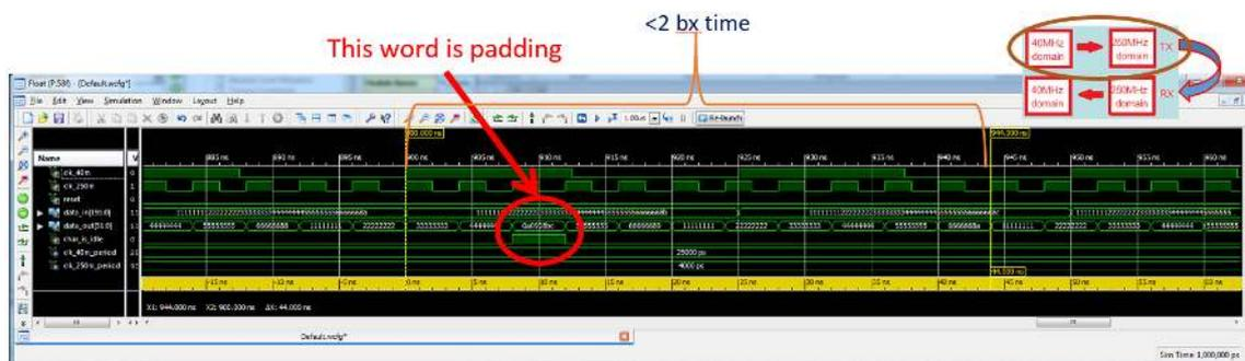
Figure F.3: TX Elastic FIFO of the asynchronous protocol 10 Gb/s, output of ISim Xilinx software [79].
