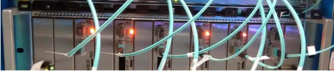
Figure C.1: Output BMTF fiber channels connected to the BMTF cards
