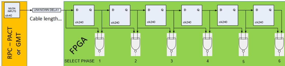
Figure 7.10: The receiver block that auto-chooses the optimum sampling phase
