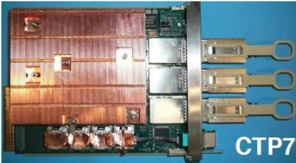
Figure 3.5: The CTP7 processor with three CXPs used in the CaloL1.
