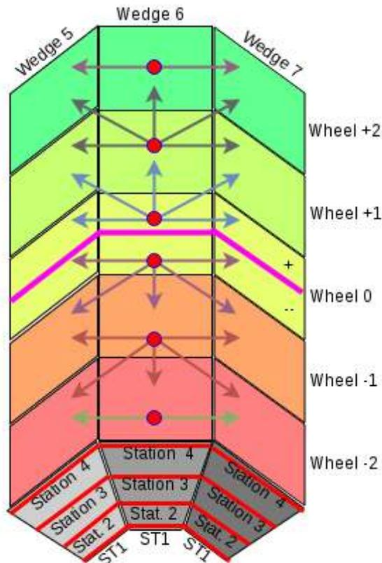
Figure 4.6: One detector muon wedge (wedge 6) in which trigger primitives are processed by 6 PHTFs (showing in red dots) in order to find possible partial muon tracks (arrows).
