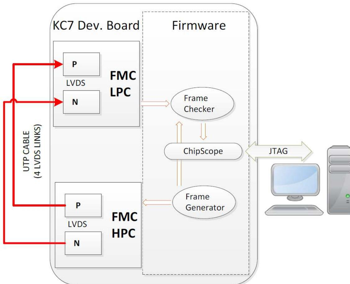
Figure A.9: Evaluation setup of copper links of EDA-02727-V1
