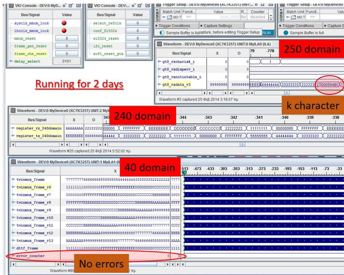
Figure F.6: Validation of the 10-Gb/s asynchronous protocol, output of Chipscope Xilinx software [81].
