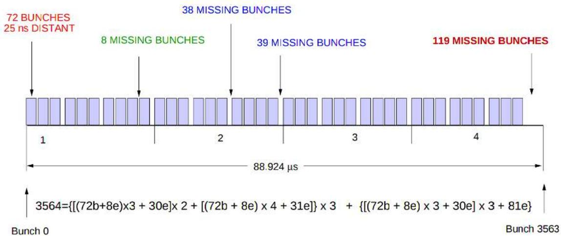
Figure 1.3: The orbit period with the 3,564 bunches in LHC. b and e indicate filled and empty bunches respectively.
