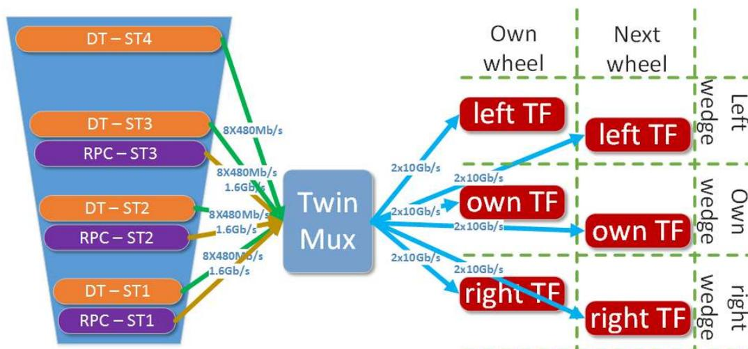
Figure 3.10: Block diagram of the TwinMux serial I/Os.
