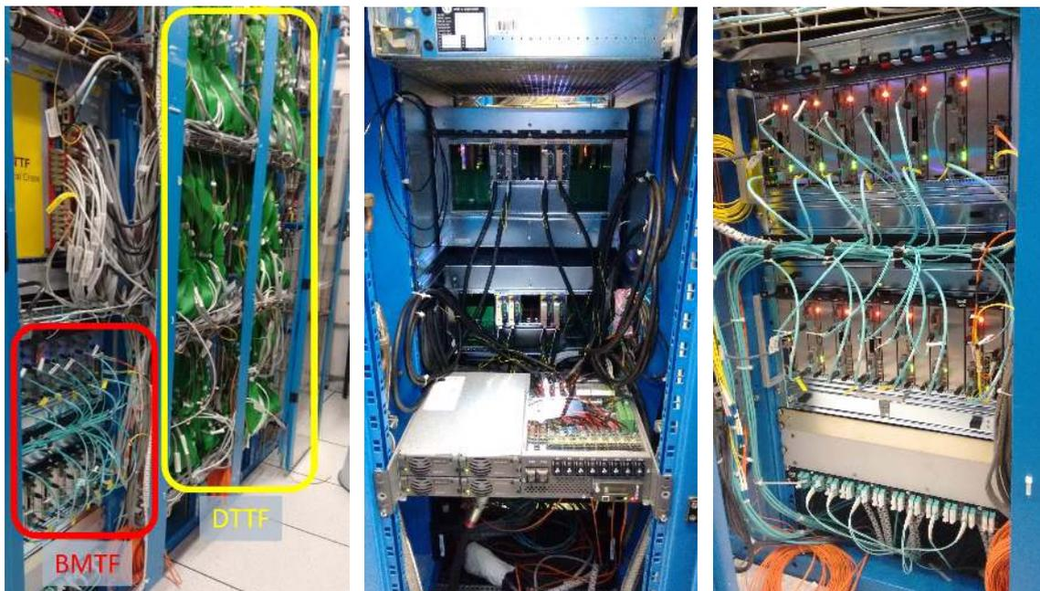
Figure 5.7: The BMTF system installed in CMS. Left: BMTF and DTTF systems. Middle: Rear side of BMTF crates. Right: Front side of BMTF crates.
