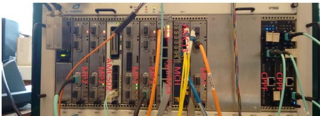
Figure 7.3:  $\mu$ TCA test-bench hosting 6 MP7s, 1 TwinMux, 2 CPPF and 1 AMC502
