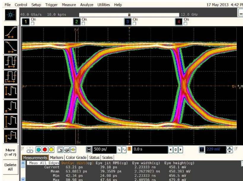
Figure A.6: Wide-open eye diagram at 400 Mb/s, indicating data transactions.
