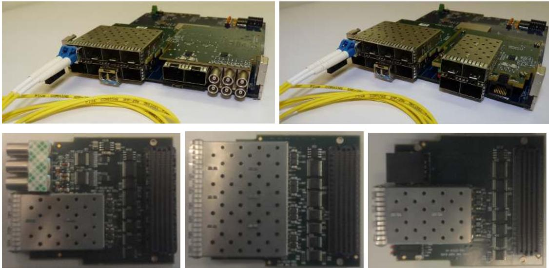
Figure A.1: Hardware used in the TCDS. Upper left: FC7 board as LPM, upper right: FC7 board as PI, down left: EDA-02708-V1 mezzanine, down middle: EDA-02707-V1 mezzanine, down right: EDA-02727-V1 mezzanine
