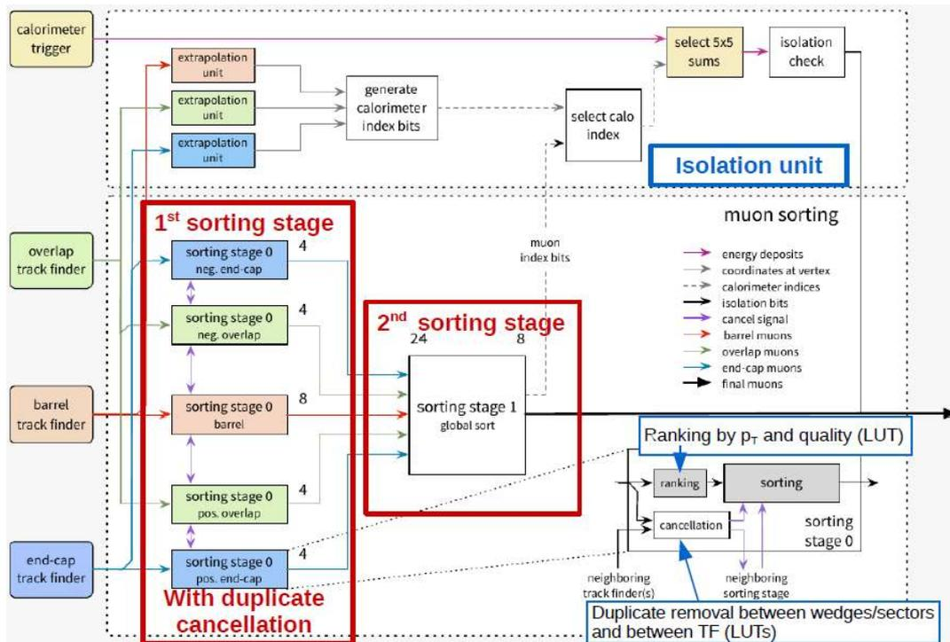
Figure 3.16: Logic block diagram of  $\mu$ GMT. The upper part shows the isolation unit and the lower part the sorting unit.
