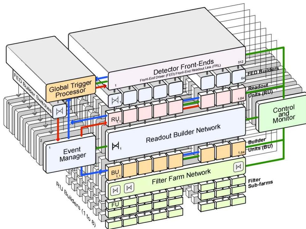
Figure 3.19: The event builder of the High Level Trigger (HLT).
