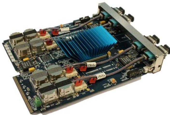
Figure 3.6: The Master Processor Virtex-7 (MP7).
