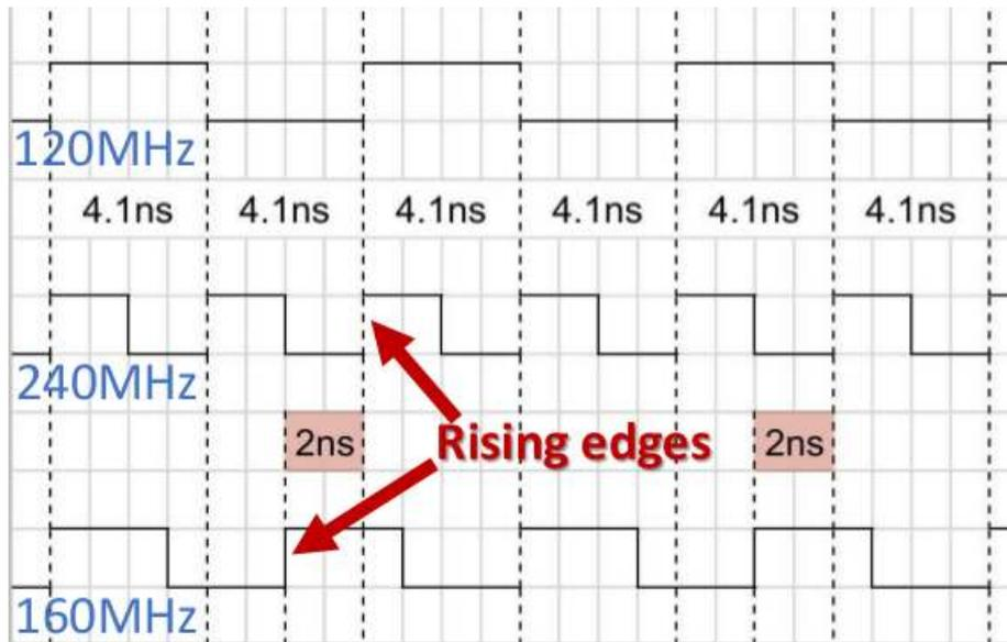
Figure 4.21: Phase difference between clock domains
