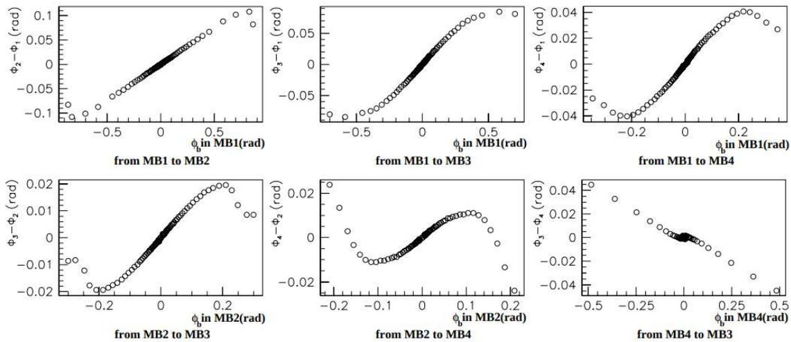
Figure 4.5: Deflection of a muon track  $\phi_{target} - \phi_{source}$ , for all Muon Station pairs as a function of the bending angle  $\phi_{b,source}$
