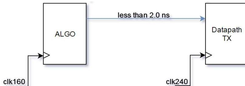
Figure 4.22: 160-MHz to 240-MHz bridge. Constrain force implementation tool to place the flip-flops close to each other.
