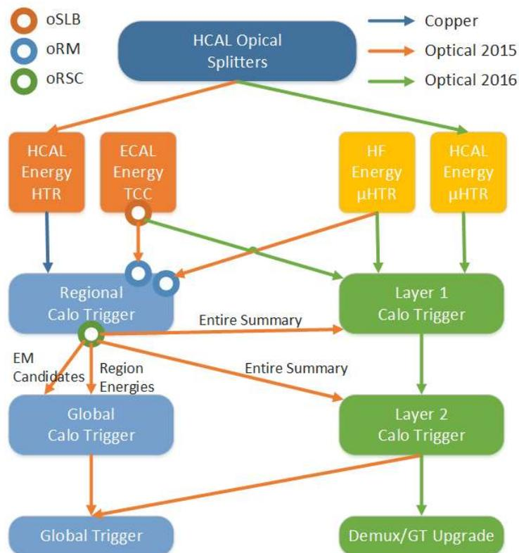
Figure 3.3: The Level-1 Calorimeter Trigger of CMS before and after the upgrade. On the left side is the old system and on the right side the upgraded system. The upgrade lasted for two years. In that period parts of the new system was getting in charge of the calorimeter trigger stage by stage.
