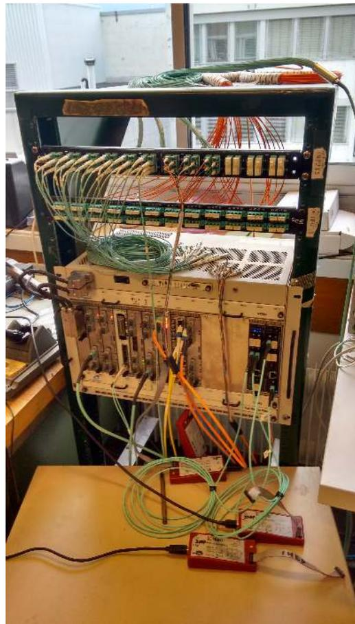
Figure 7.1: Electronics setup for the testing of the TwinMux, CPPF and AMC502
