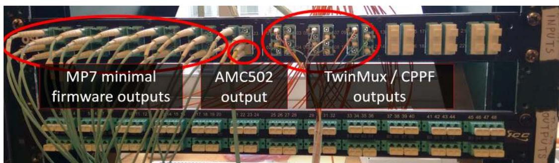
Figure 7.2: Patch panel connections of MP7, TwinMux, CPPF and AMC502 cards
