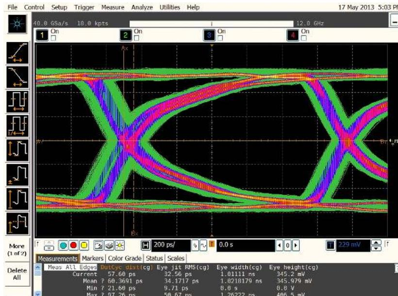
Figure A.7: Open eye diagram at 800 Mb/s, indicating safe data transactions.
