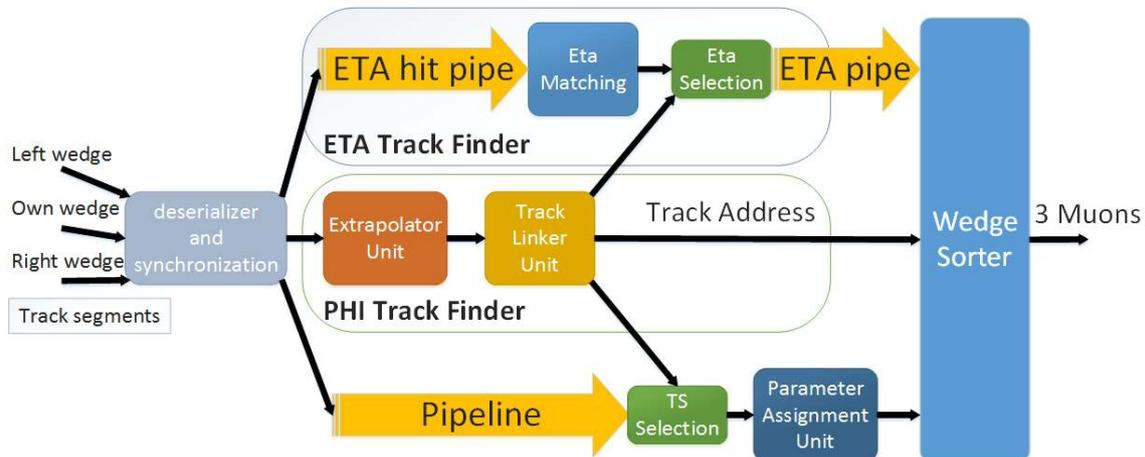
Figure 4.2: Block diagram of the track finder algorithm.
