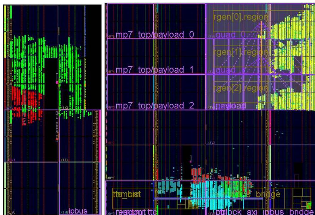
Figure 7.5: Post-implementation floor plan of the CPPF card FPGAs: Left Control Kintex-7, right: Core Virtex-7
