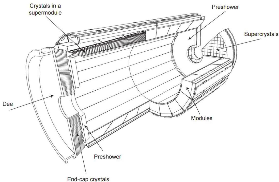
Figure 2.6: The layout of ECAL
