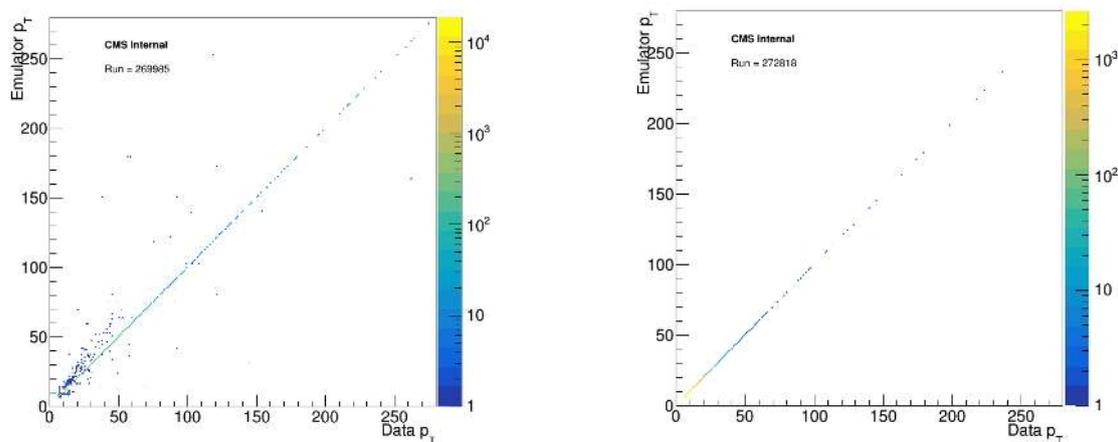
Figure 5.9: Fixing  $p_T$  corruption. On the left-hand-side plot the effect of corrupted data is shown. On the right-hand-side plot the symptom is gone.
