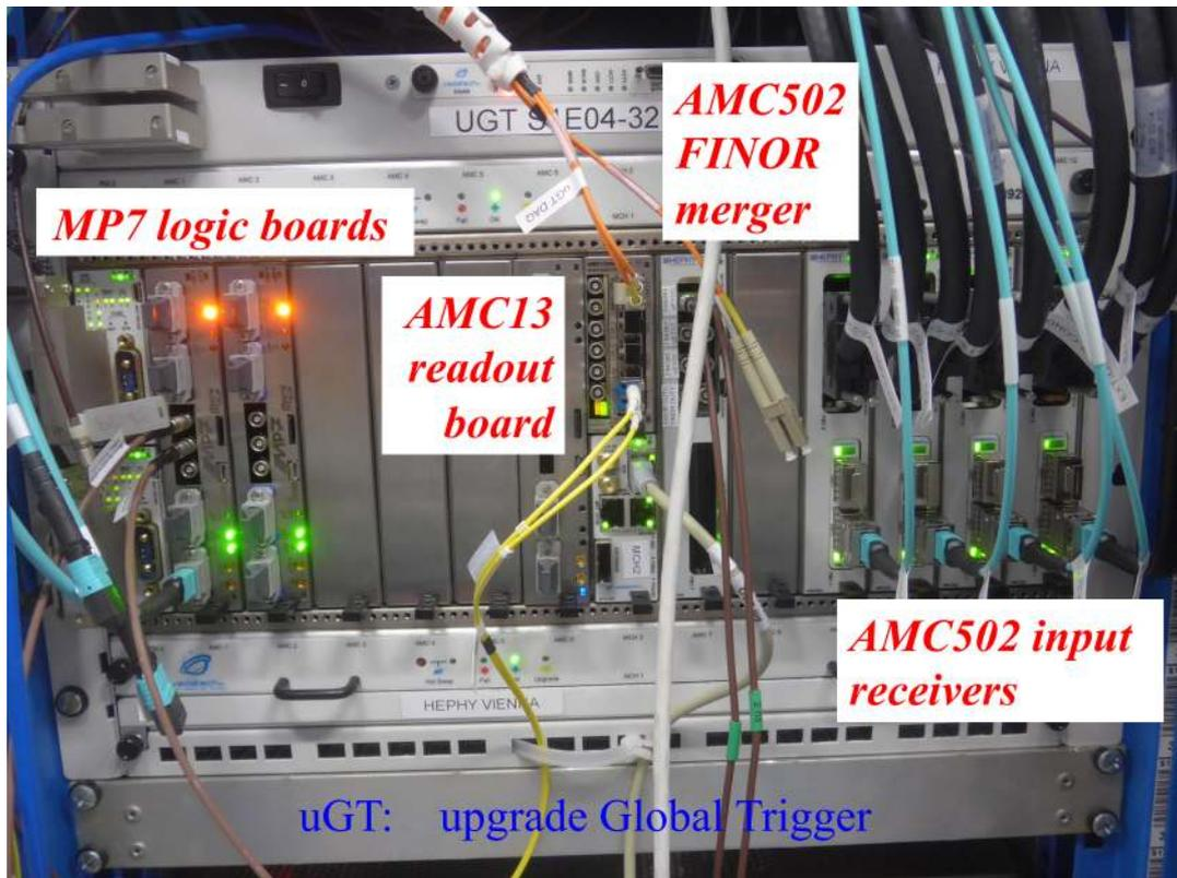
Figure 3.18: The  $\mu$ GT crate. From left to right the crate hosts two power modules, three MP7s (the first two are operational), one AMC13, one MCH and five AMC502 (the first generates the finalOR and the other four convert LVDS signals to 10-Gb/s asynchronous optical links).
