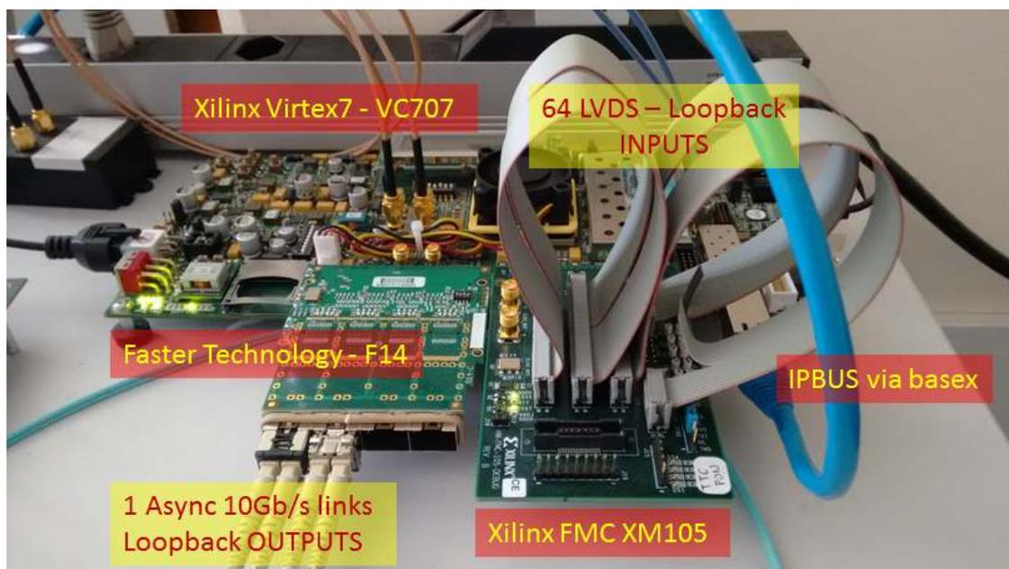
Figure 7.9: VC707 - Developing fallback for the muon trigger
