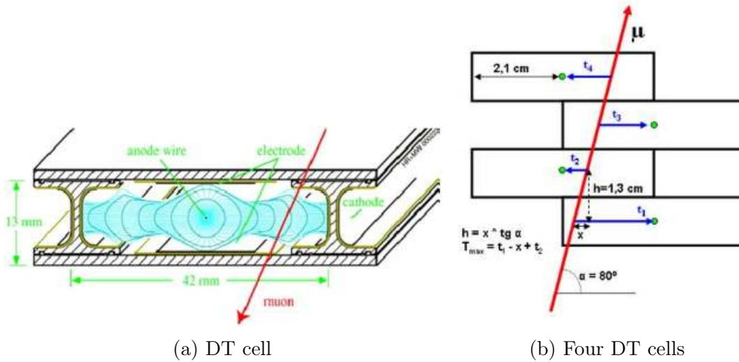
Figure 2.9: Drift Tubes cell ionised by a muon
