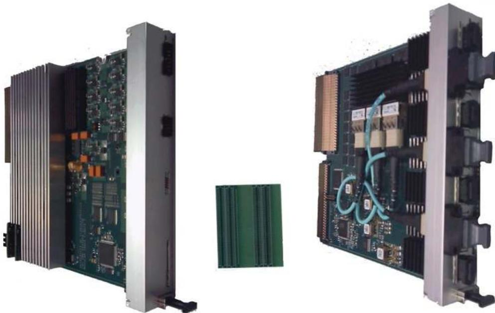
Figure 3.14: MTF7 dual board. On the left side is the optical board with the I/O links. On the right is the base board that hosts the virtex-7 Core FPGA. These are interconnected by a custom backplane (center).
