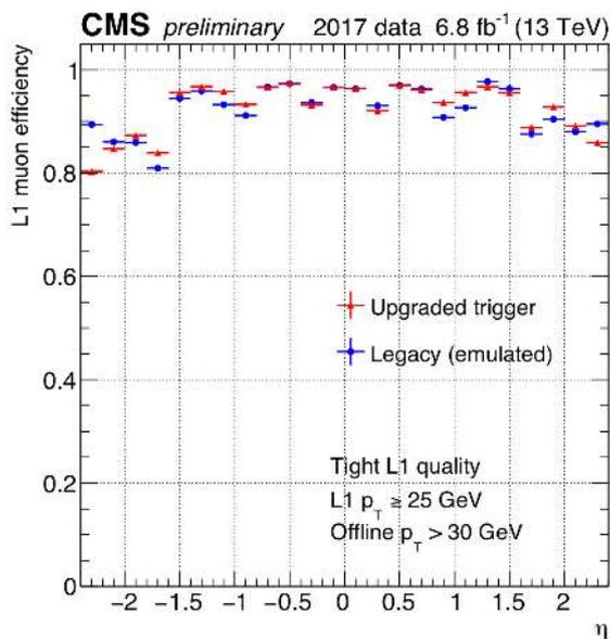
Figure 5.16: Barrel (BMTF) and legacy (DTTF) single Muon efficiency versus  $\eta$ .
