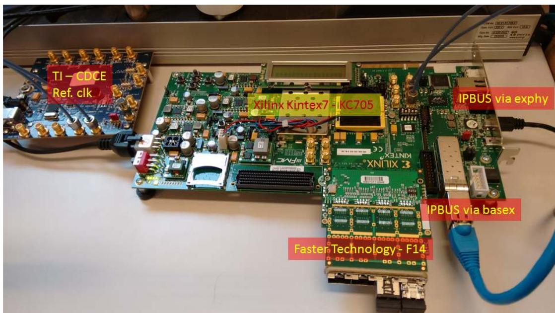
Figure 7.8: KC705 - Developing fallback for the muon trigger
