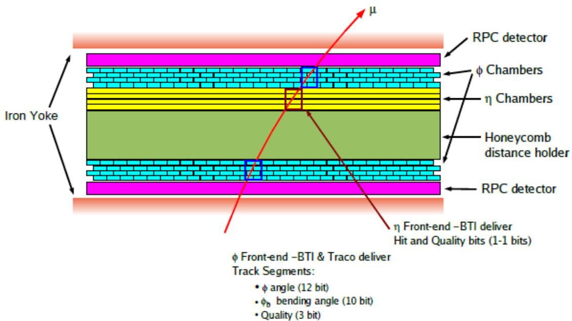
Figure 2.10: DT layers and superlayers in a DT detector
