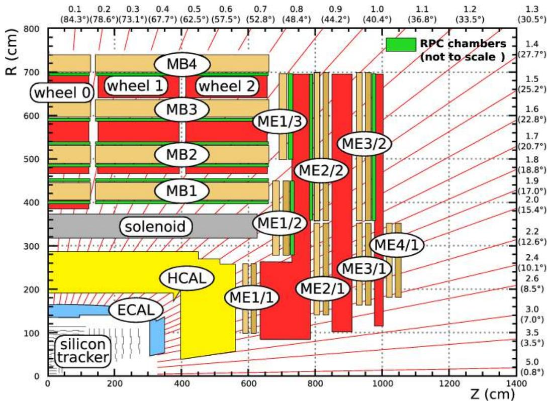
Figure 2.12: Schematic view of one quarter of CMS, in the  $z$ - $\phi$  plane. RPC chambers appear with green color
