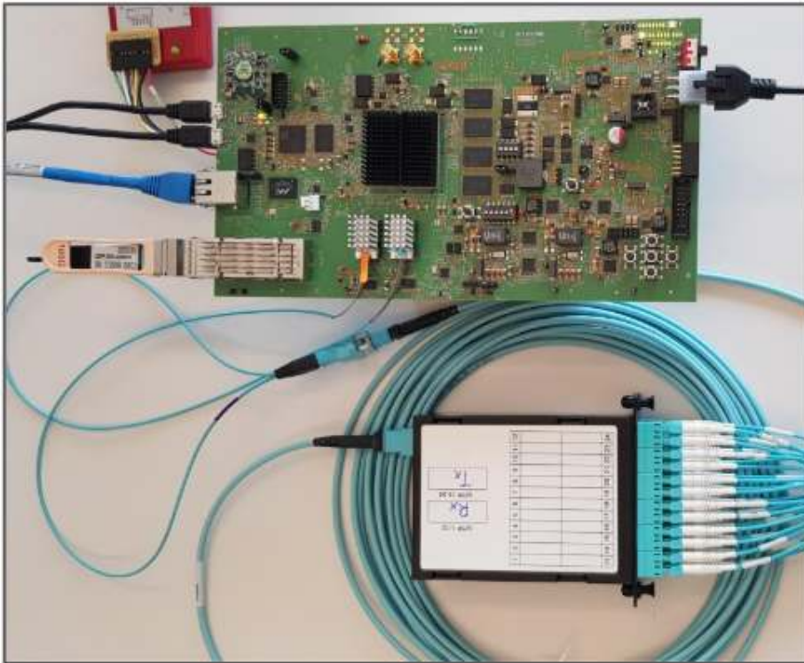
Figure 7.26: The optical loopback test configuration used to test the Hermes links. Three MGT quads (12 transceivers) are routed to the Firefly optical modules. The 12 optical transmitter fibers and 12 optical receiver fibers, coming from the Firefly optical engines, are merged in a 10 m long MTP cable with 24 fibers. An MTP-to-LC cassette is used, to split the fibers and forward the transmitters to the corresponding receivers, creating a 20 m optical loopback path.
